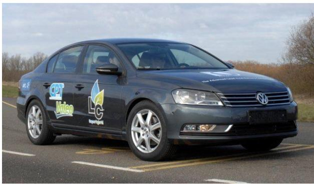
LC Super Hybrid technology demonstrator is based on a VW Passat 1.4-litre TSI model
