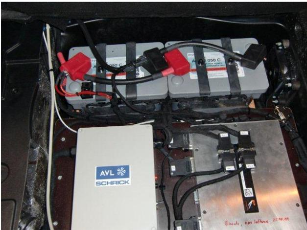
LC Super Hybrid lead-carbon battery installation and test equipment
