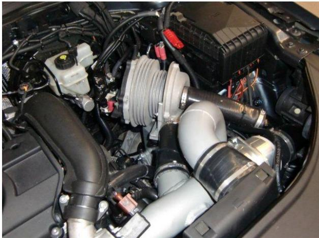
LC Super Hybrid features a Valeo electric supercharger which boosts the existing turbocharger
