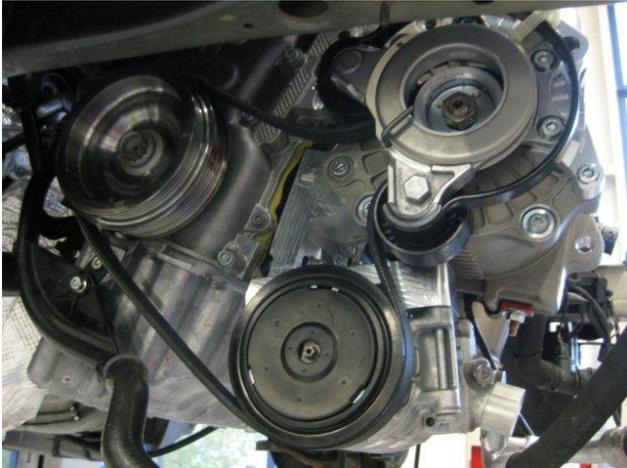
LC Super Hybrid features CPT SpeedStart stop-start technology (top right) and Mubea belt tensioner
